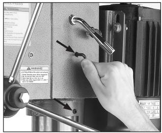
Figure 14. Securing headstock to column.
